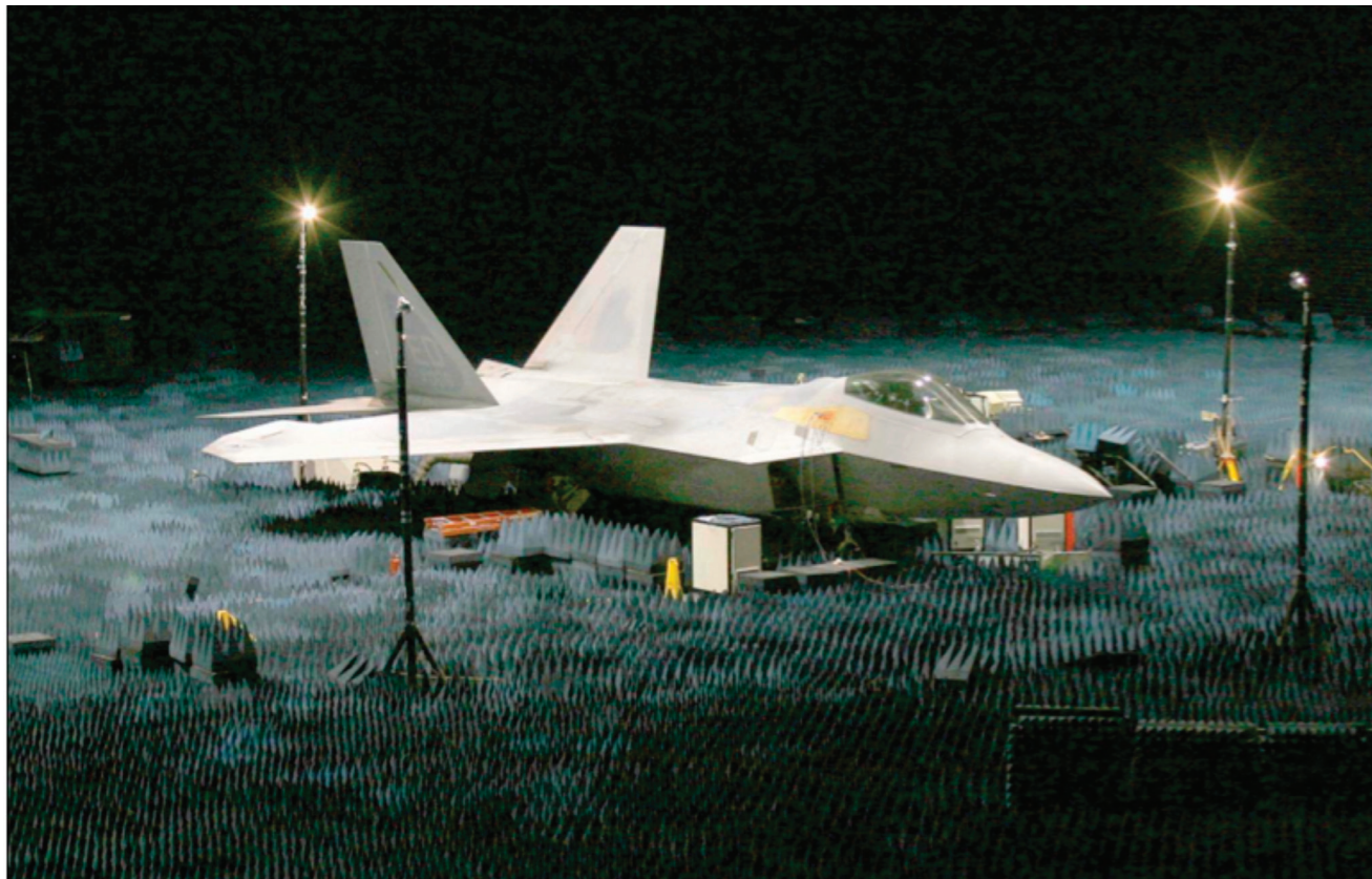
Various methods, such as anechoic chambers, are used to test the effectiveness of ECMs.
